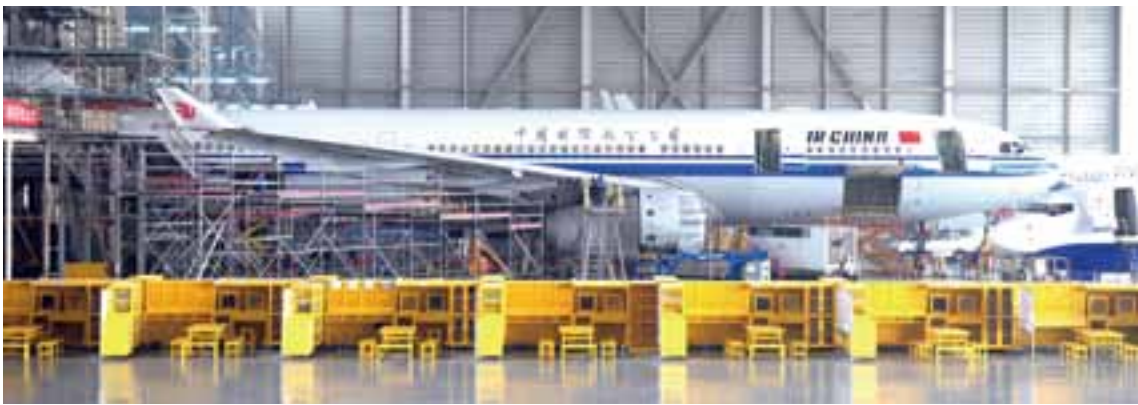
Ameco overhaul workstation comprises seven semi-enclosed areas with different functions. This centralises the aircraft overhaul resources that used to be scattered in different locations and provides mechanics with one-stop support, thus improving work efficiency and creates more effective work hours
