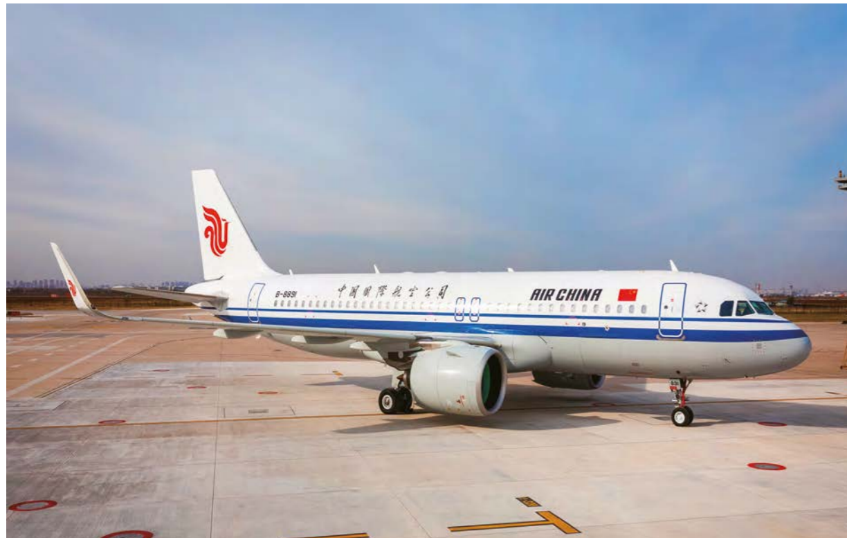
Airbus 320NEO used the new generation of PW1100G/LEAP-1A engine with larger engine fan and was equipped with the new generation of Sharklet to increase the safety margin of flights
